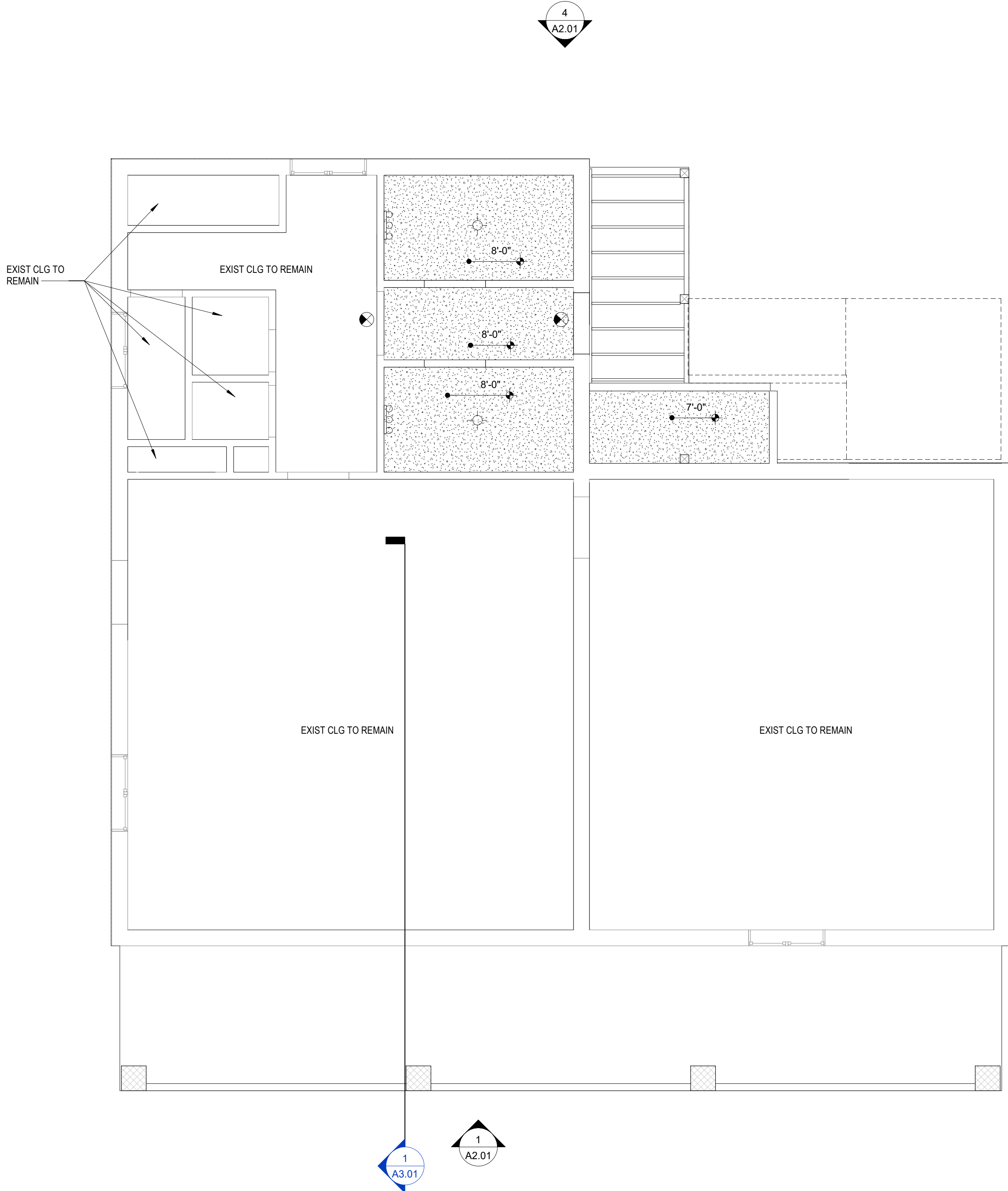
FIRST FLOOR REFLECTED CEILING PLAN 2 A1.02 1/4" = 1'-0"
